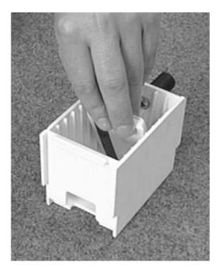
Drop the cards flat down into the plastic Cassette, side to be printed uppermost, mag stripe to the left and facing down (if used).
